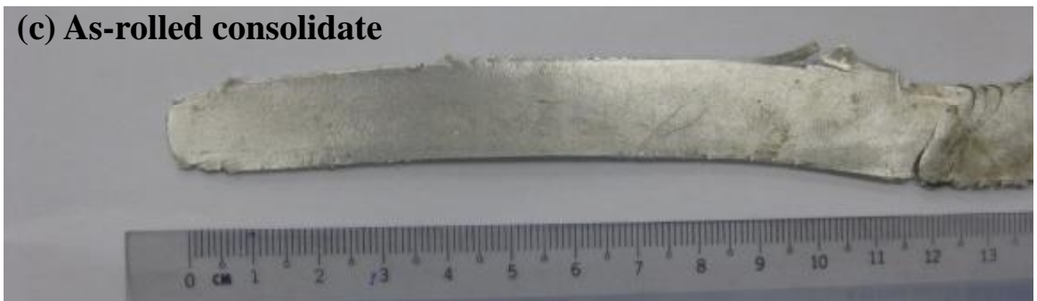
Figure 4-4. Photographs of the consolidated samples: (a) as-sintered consolidate; (b) as-extruded consolidate; and (c) as-rolled consolidate.
